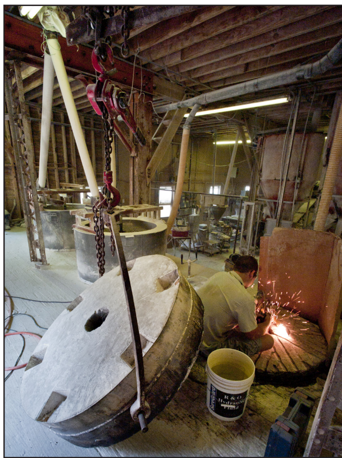
Ray is seen here by the millpond and inside the mill with one of his grandsons. A millstone is seen lifted from its position for repair of shaft on which the upper stone rotates.
