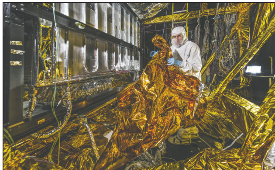
Thermal blankets are prepared for testing the telescope in the vacuum chamber.
