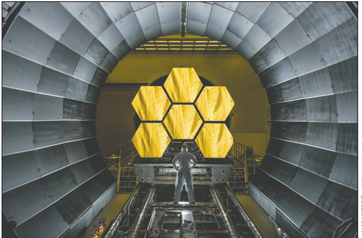
The first six of 18 mirrors of the Webb Telescope are prepared for cryogenic testing.
